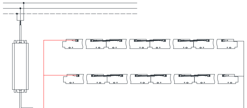
HLG-120-48A for 4S x 2P =8pcs LED module 4S=51.5V @ 1.25A 64W X 2P =128W 13100Lm AC Power 140W PF0.9
