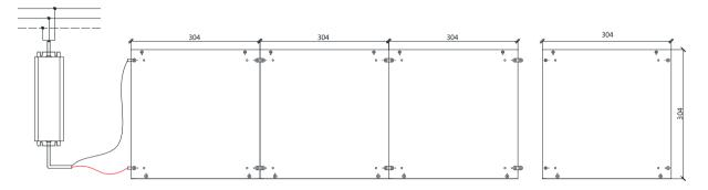
1, Maximum series connected power 240W. (24V 10A)
