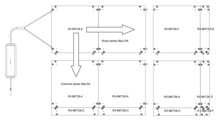
Note: Row and column totals; must be less than the number of LED module can be spliced (Row x Column ≤ 10A 240W)
