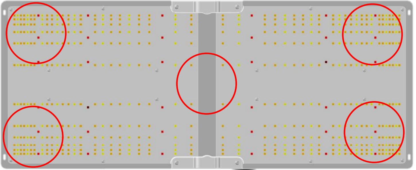
Optimized LED arrangement, high-density arrangement at four corners, sparse center, improve illumination uniformity
