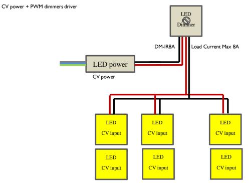
Calculations are based on 85% max load on Constant voltage power supply
