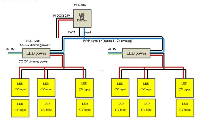
A large area of simple synchronous dimming system - No PWM flicker  $\,$
