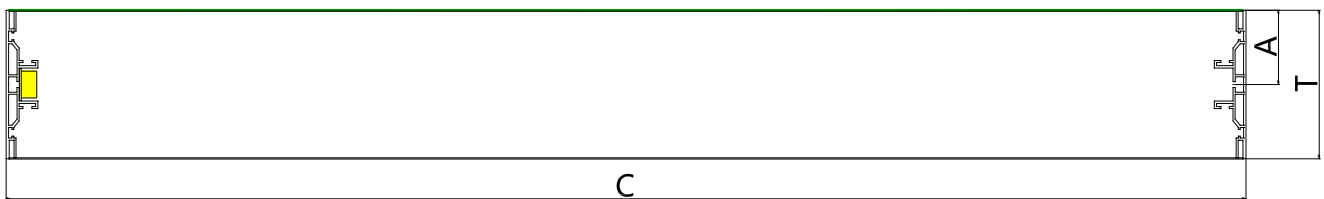
One-sided Lighting (1x2m light box only one LED module)
